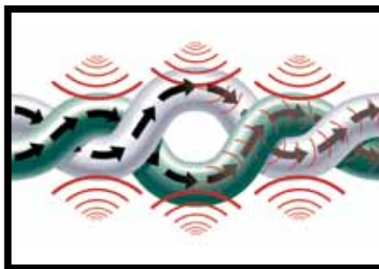
Illustration 1: Example of Non-Bonded Pair. As cable is stretched and pulled, pairs begin to separate, causing a degradation in signal quality.
